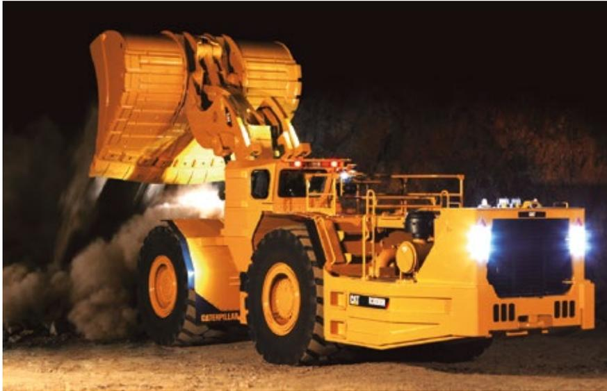
◀ LAS NUEVAS SERIES DE CARGADORES DE BAJO PERFIL CAT, EN SUS DIVERSOS MODELOS, INCORPORAN EL SISTEMA VENTILATION REDUCTION (VR), QUE OPTIMIZA LA MEZCLA AIRE- COMBUSTIBLE Y REDUCE LOS NIVELES DE EMISIONES.
